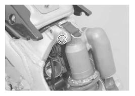
· Remove the rear shock absorber lower mounting bolt and nut. NOTE:
