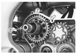
• Remove the following parts from the kick starter shaft 9.
