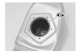
• When installing the fuel pump assembly, first tighten all the fuel pump mounting bolts lightly and then to the specified torque.
