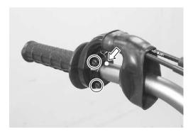
• Slightly loosen the handlebar holder set nuts.
