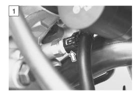
5) Insert the needle-point probes to the lead wire coupler.
