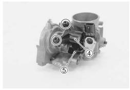
• Remove the fuel injector ⑤ from the fuel pipe ④.
