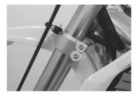
• Tighten the fork cylinder unit (LH) or air cylinder unit (RH) to the specified torque.
