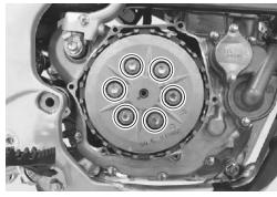
• Remove the clutch pressure plate ②, bearing ③ and push piece ④.
