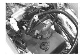
Connect a new spark plug to spark plug cap and ground it to the cylinder head.
