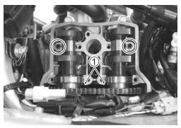
Apply grease to the new O-ring and install it to the camshaft journal holder.
