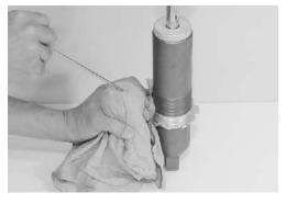
• Remove the compression adjuster assembly ① with the special tool from the rear shock absorber.
