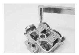
· Remove the camshaft journal holder, and read the width of the compressed plastigage with envelope scale. This measurement should be taken at the widest part.
