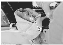
• Remove the dust boot 4 and snap ring 5.
