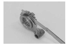
• Measure the gearshift fork thickness with a vernier calipers.
