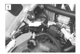
4) Disconnect the CKP sensor coupler and measure the resistance.
