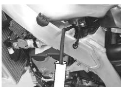
• Connect the proper lead wires into the fuel pump coupler (fuel pump side) and apply 12 volts to the fuel pump (between terminal (A) and terminal (B) for 10 seconds and measure the amount of fuel discharged.
