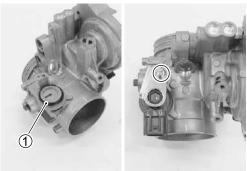
Apply thin coat of engine oil to new O-ring ② and new cushion seal ③.
