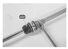
Clamp the flat part of axle holder with a vise. Protect the axle holder with a rag when using a vise.
