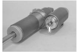
· Press the valve with a screwdriver.
