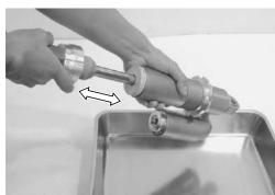
Pour the fresh specified rear suspension oil as shown while moving the rod.
