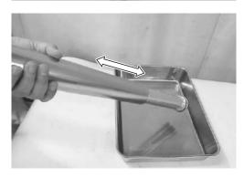
• Hold the front fork inverted position for more than 20 minutes to allow the fork oil to fully drain.
