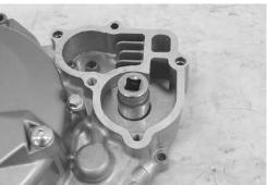
• Check engine oil flow before installing the water pump shaft.
