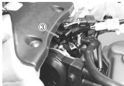
• Remove the throttle cable cover 4.
