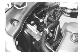
4) Disconnect the injector coupler and measure the resistance between terminals.
