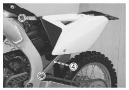
• Remove the rear shock absorber upper mounting bolt and nut.
