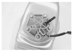
• Connect the fuel hose to the fuel pump securely. ( 13-3)
