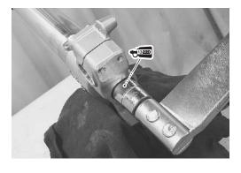
• Loosen and remove the fork cylinder unit from the outer tube and slowly slide down the outer tube.
