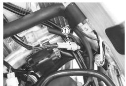
Measure the engine stop switch resistance between B/Y lead wire and B/W lead wire.
