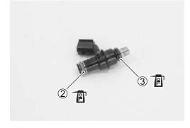
• Install the fuel injector by pushing it straight to fuel pipe.
