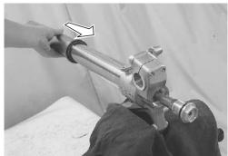
Hold the lock-nut ④ with a wrench and remove the center bolt
