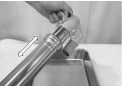
• Clamp the flat part of axle holder 4 with a vise. Protect the axle holder 4 with a rag when using a vise.
