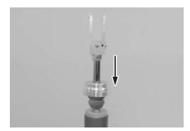
• Evenly hammer the stopper 1 with a screwdriver or equivalent and remove it from the rear shock absorber body.
