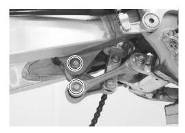
• Remove the swingarm pivot nut and washer.
