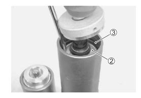
• Remove the circlip 3.
